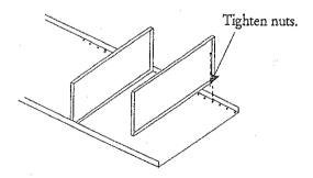
Shelf bolts are installed from the back and through the post and back and tighten nuts finger tight.
