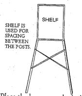
Place the braces on the inside of the post. Insert ¼ x ½ long bolts from the outside of the posts. Attach nuts and tighten.
