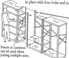
For fastening units together, use 1" bolts and nuts.
